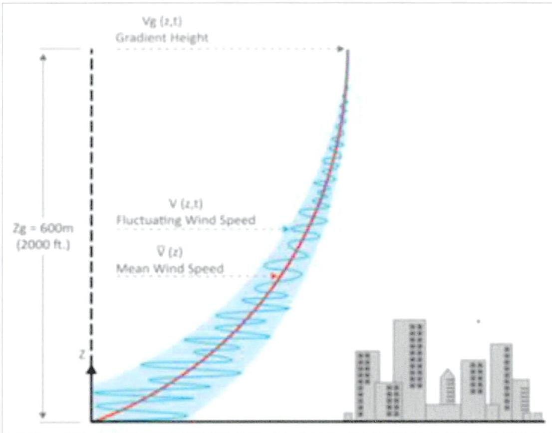
**Figure 11-3: Atmospheric wind velocity profile**
