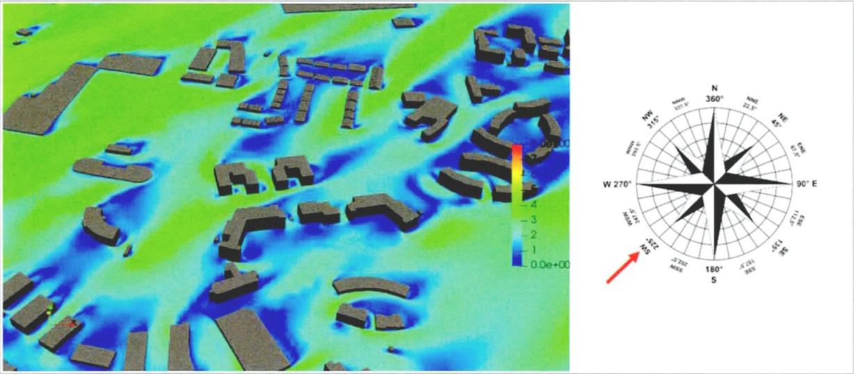
Figure 11-24: Pedestrian Level - Velocity Results at 1.5m above the ground - Wind Direction: 225°
