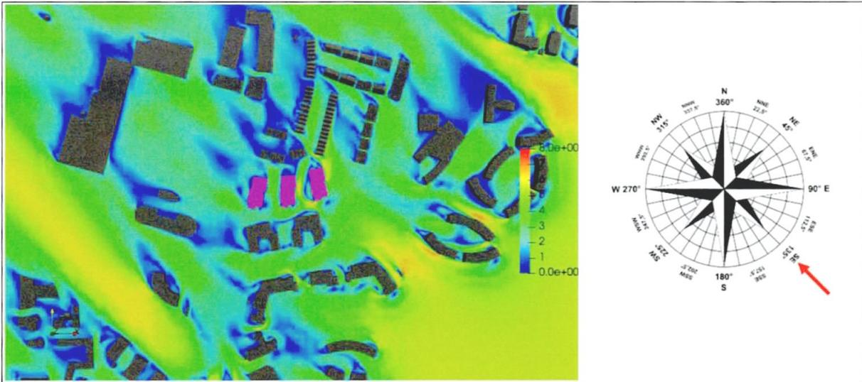
Figure 11-35: Pedestrian Level - Velocity Results at 1.5m above the ground - Wind Direction: 135°
