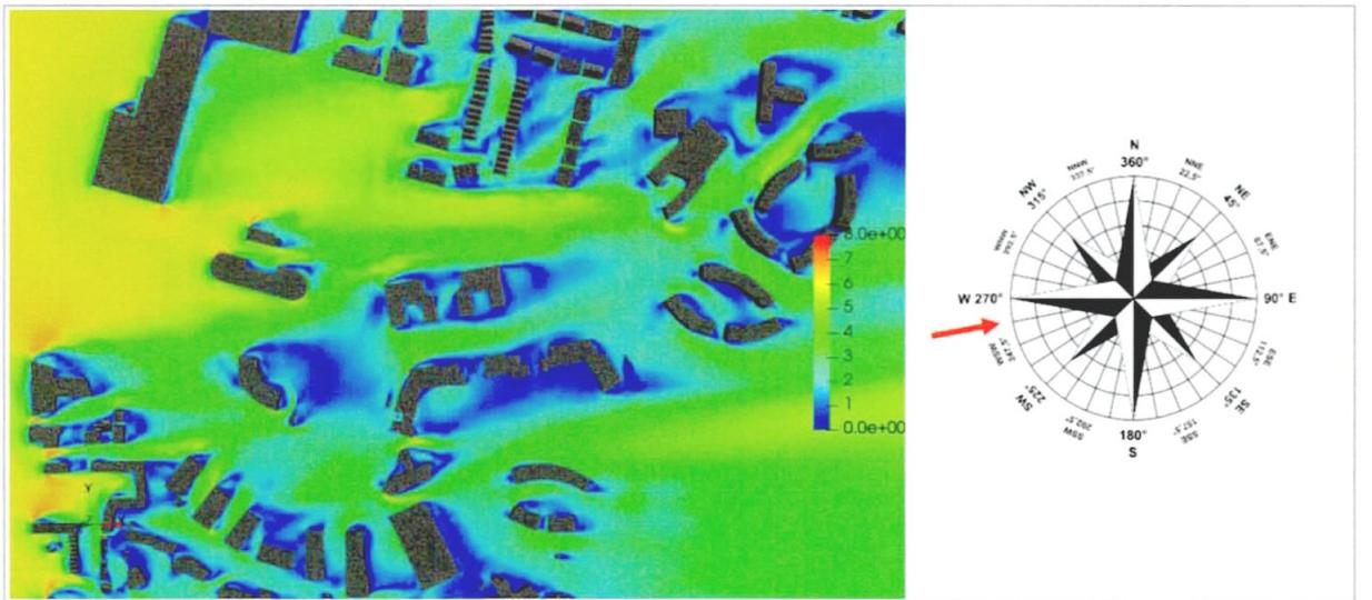
Figure 11-19: Pedestrian Level - Velocity Results at 1.5m above the ground - Wind Direction: 258°
