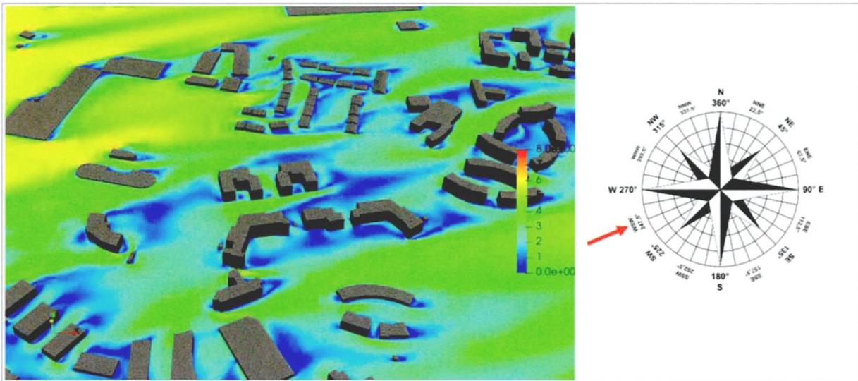
Figure 11-26: Pedestrian Level - Velocity Results at 1.5m above the ground - Wind Direction: 247°
