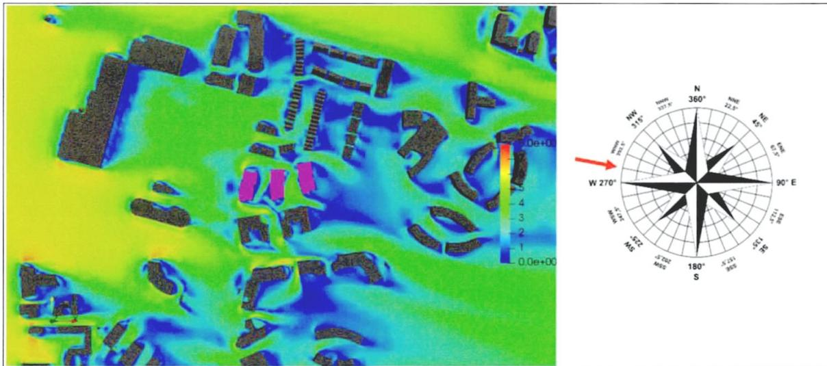
Figure 11-44: Pedestrian Level - Velocity Results at 1.5m above the ground - Wind Direction: 281°
