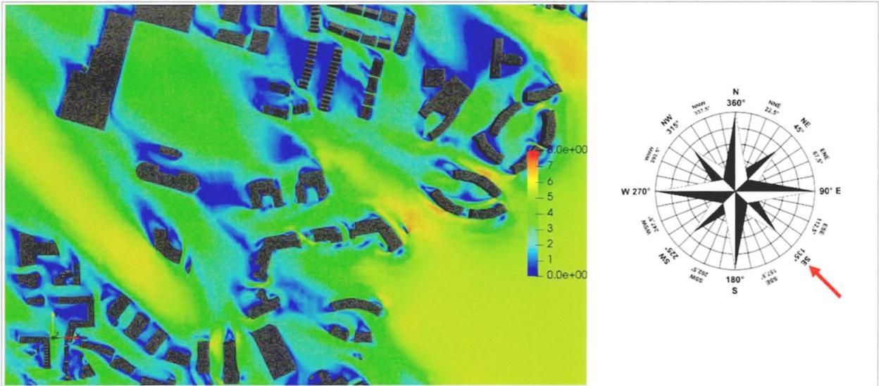
Figure 11-15: Pedestrian Level - Velocity Results at 1.5m above the ground - Wind Direction: 135°
