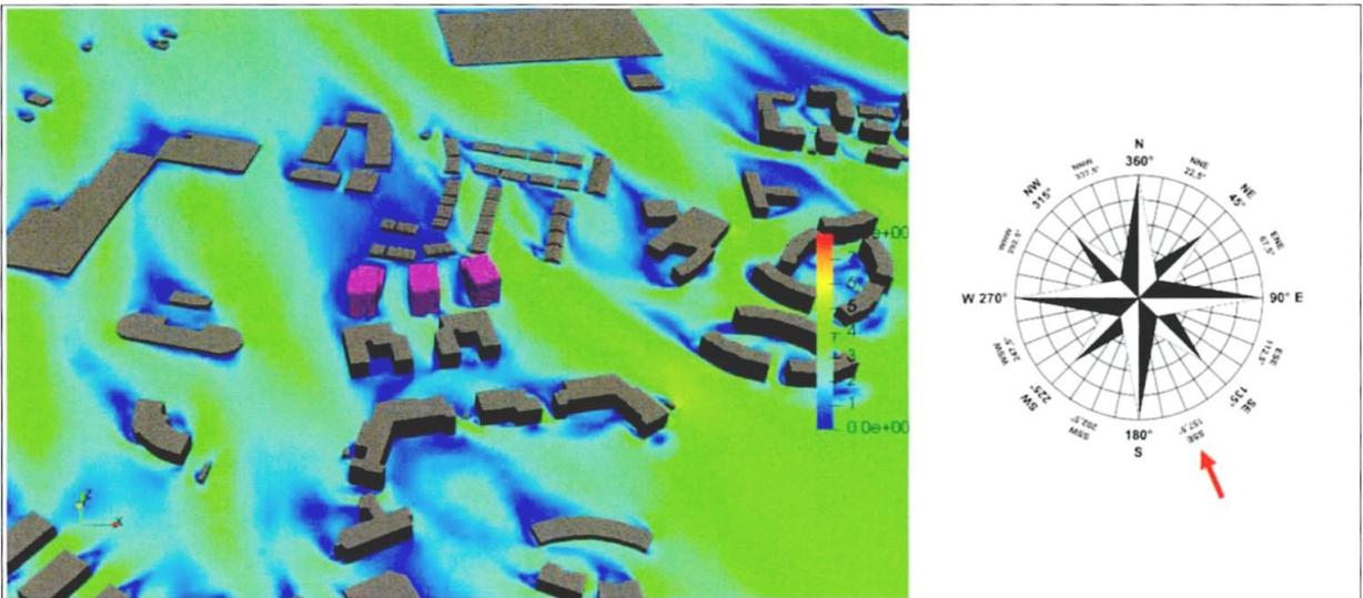
Figure 11-48: Pedestrian Level - Velocity Results at 1.5m above the ground - Wind Direction: 157°
