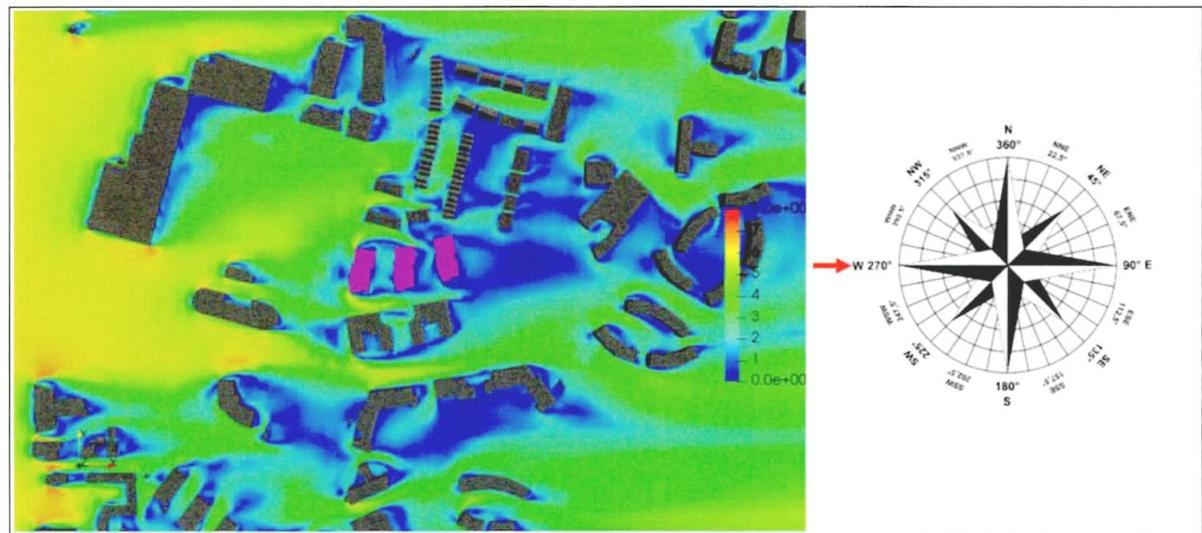
Figure 11-43: Pedestrian Level - Velocity Results at 1.5m above the ground - Wind Direction: 270°
