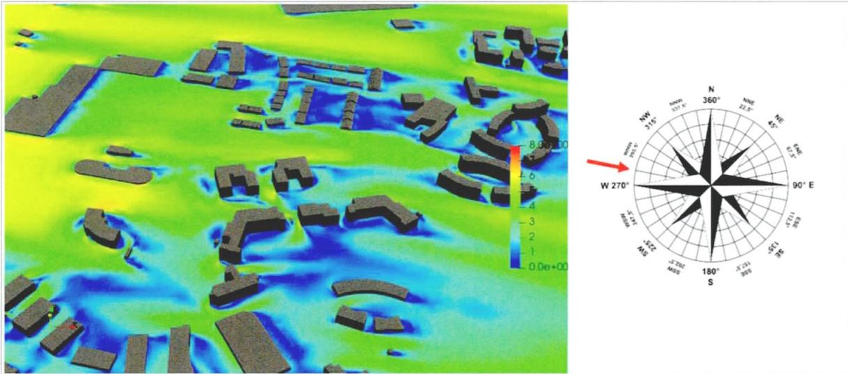
Figure 11-29: Pedestrian Level - Velocity Results at 1.5m above the ground - Wind Direction: 281°
