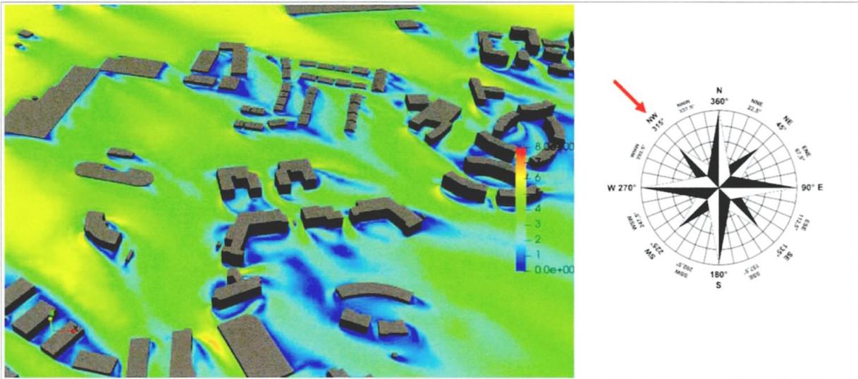
Figure 11-30: Pedestrian Level - Velocity Results at 1.5m above the ground - Wind Direction: 315°
