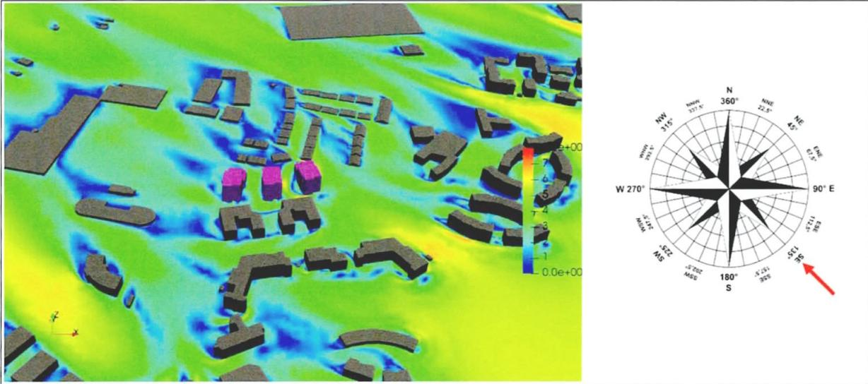
Figure 11-47: Pedestrian Level - Velocity Results at 1.5m above the ground - Wind Direction: 135°
