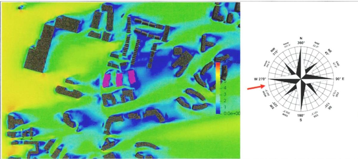
Figure 11-42: Pedestrian Level - Velocity Results at 1.5m above the ground - Wind Direction: 258°
