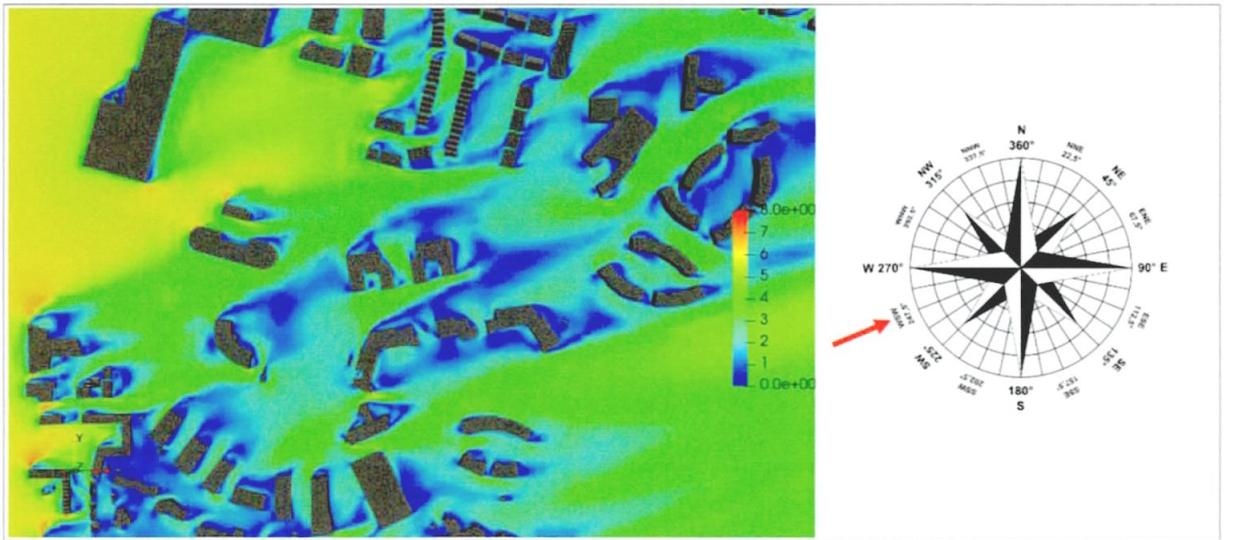
Figure 11-18: Pedestrian Level - Velocity Results at 1.5m above the ground - Wind Direction: 247°
