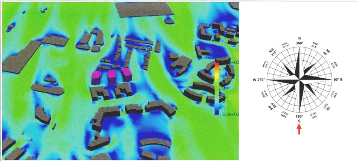
Figure 11-49: Pedestrian Level - Velocity Results at 1.5m above the ground - Wind Direction: 180°
