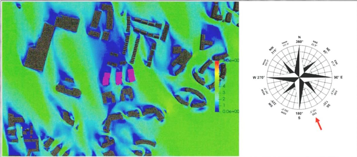
Figure 11-36: Pedestrian Level - Velocity Results at 1.5m above the ground - Wind Direction: 157°
