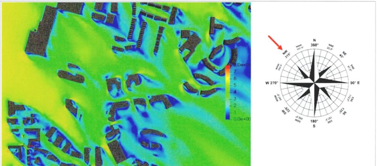
Figure 11-22: Pedestrian Level - Velocity Results at 1.5m above the ground - Wind Direction: 315°
