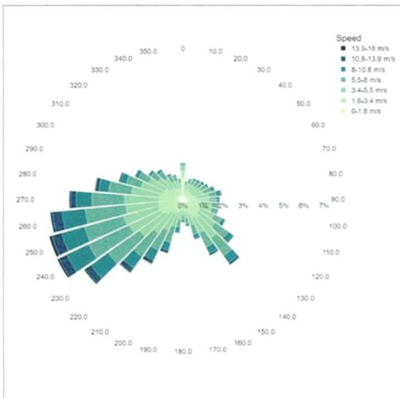
, presents the wind speed diagram for Dublin, the diagram shows how often (how many days per month) the wind blows with a specific speed.
