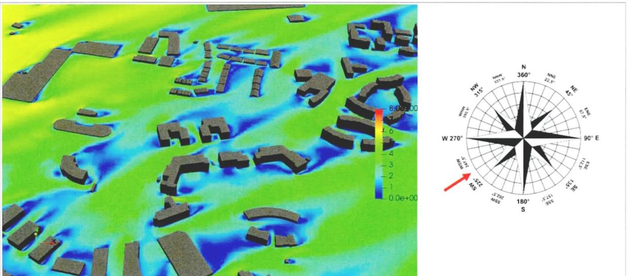
Figure 11-25: Pedestrian Level - Velocity Results at 1.5m above the ground - Wind Direction: 236°
