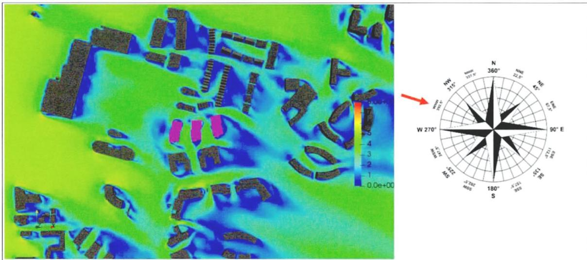
Figure 11-45: Pedestrian Level - Velocity Results at 1.5m above the ground - Wind Direction: 292°
