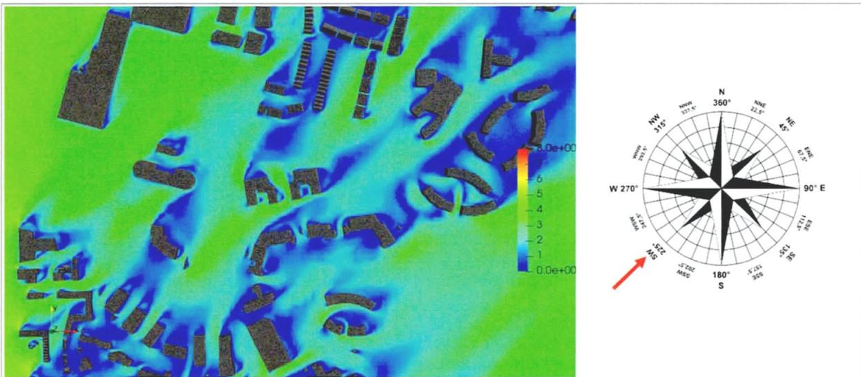
Figure 11-16: Pedestrian Level - Velocity Results at 1.5m above the ground - Wind Direction: 225°
