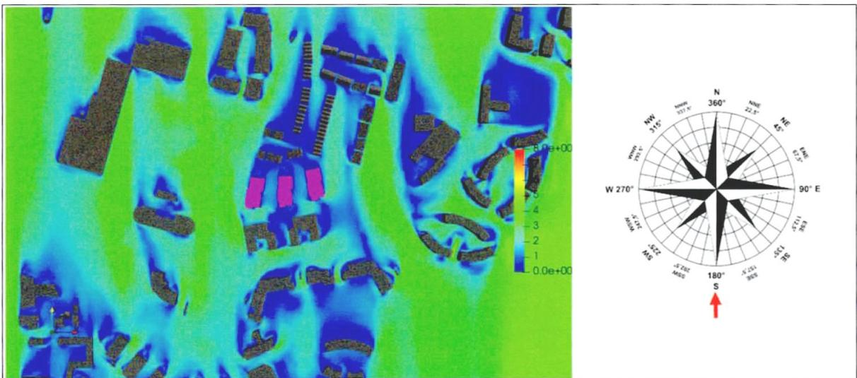
Figure 11-37: Pedestrian Level - Velocity Results at 1.5m above the ground - Wind Direction: 180°
