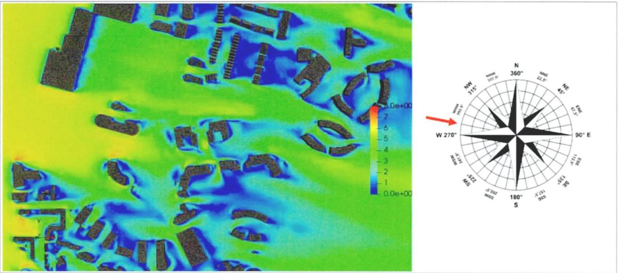
Figure 11-21: Pedestrian Level - Velocity Results at 1.5m above the ground - Wind Direction: 281°
