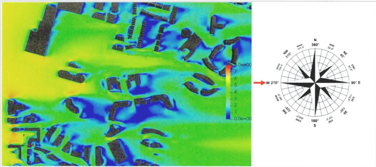
Figure 11-20: Pedestrian Level - Velocity Results at 1.5m above the ground - Wind Direction: 270°
