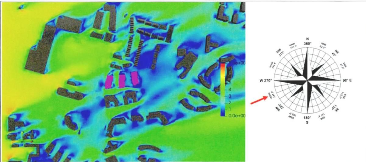
Figure 11-41: Pedestrian Level - Velocity Results at 1.5m above the ground - Wind Direction: 247°
