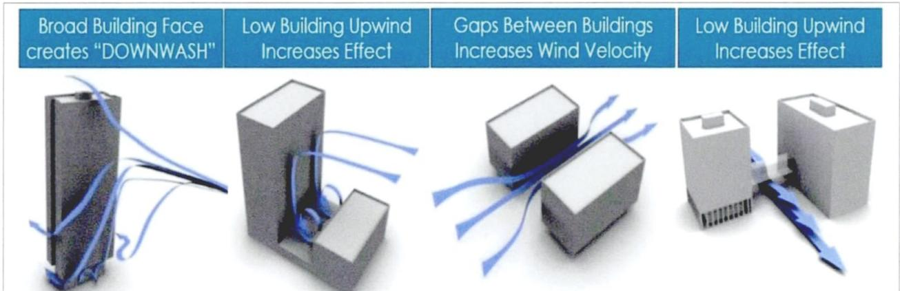
**Figure 11-4: Wind patterns created around buildings showing typical wind microclimate in an urban context**
