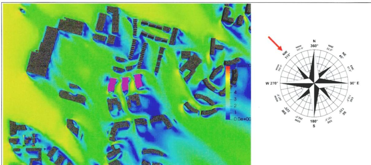
Figure 11-46: Pedestrian Level - Velocity Results at 1.5m above the ground - Wind Direction: 315°
