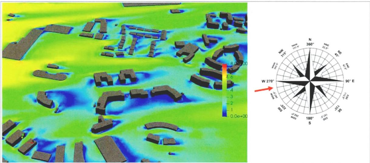
Figure 11-27: Pedestrian Level - Velocity Results at 1.5m above the ground - Wind Direction: 258°
