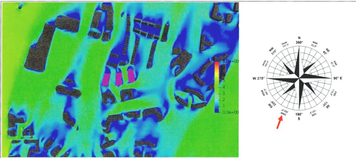
Figure 11-38: Pedestrian Level - Velocity Results at 1.5m above the ground - Wind Direction: 202°
