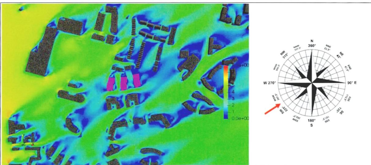
Figure 11-40: Pedestrian Level - Velocity Results at 1.5m above the ground - Wind Direction: 236°
