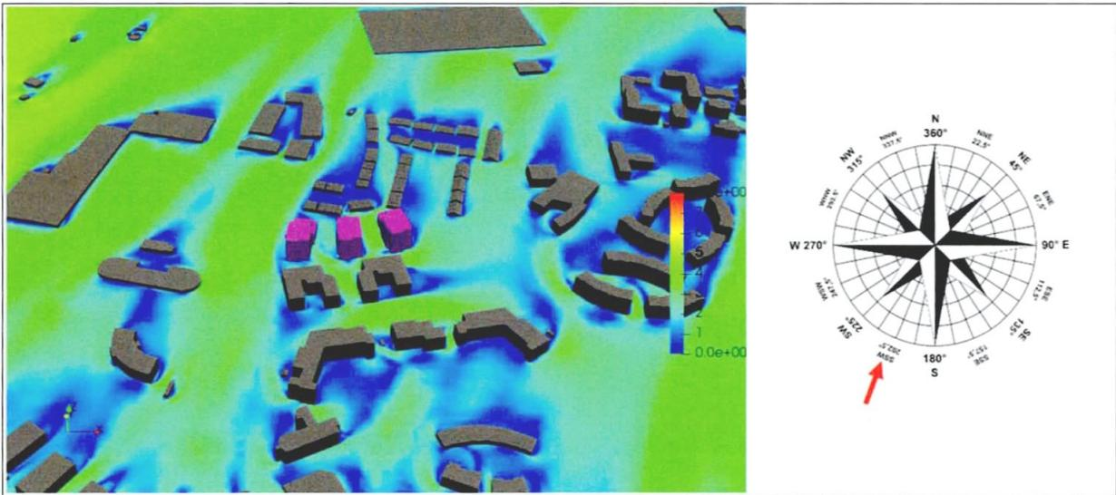
Figure 11-50: Pedestrian Level - Velocity Results at 1.5m above the ground - Wind Direction: 202°
