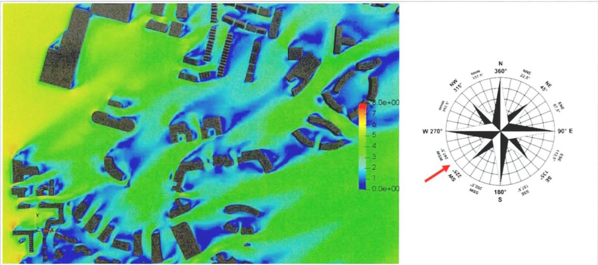
Figure 11-17: Pedestrian Level - Velocity Results at 1.5m above the ground - Wind Direction: 236°
