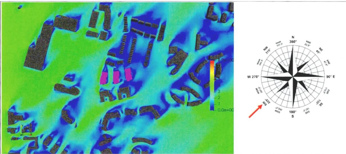
Figure 11-39: Pedestrian Level - Velocity Results at 1.5m above the ground - Wind Direction: 225°
