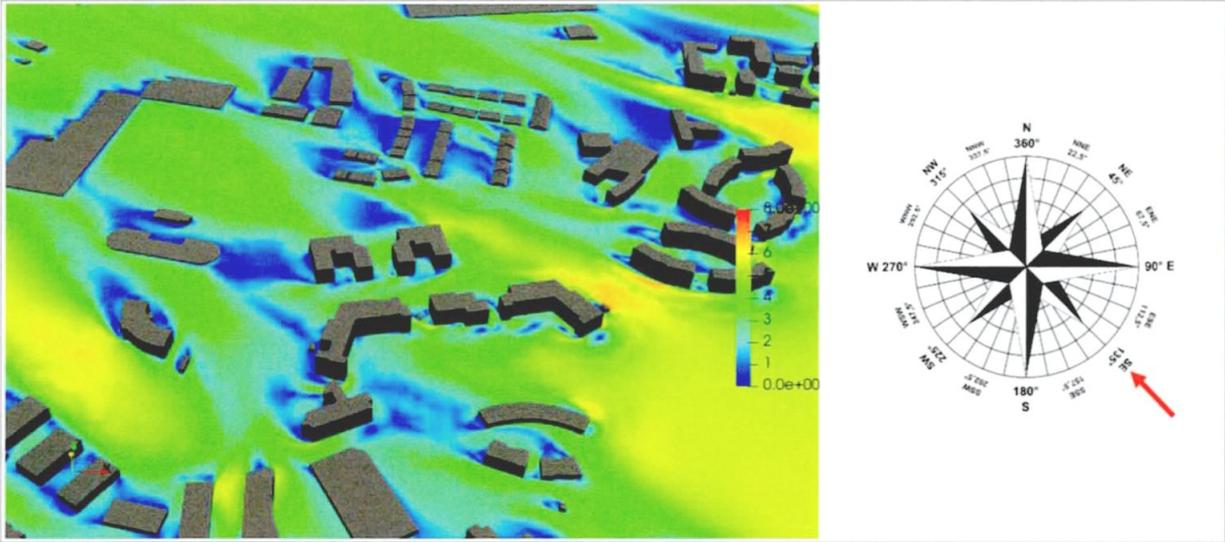
Figure 11-23: Pedestrian Level - Velocity Results at 1.5m above the ground - Wind Direction: 135°
