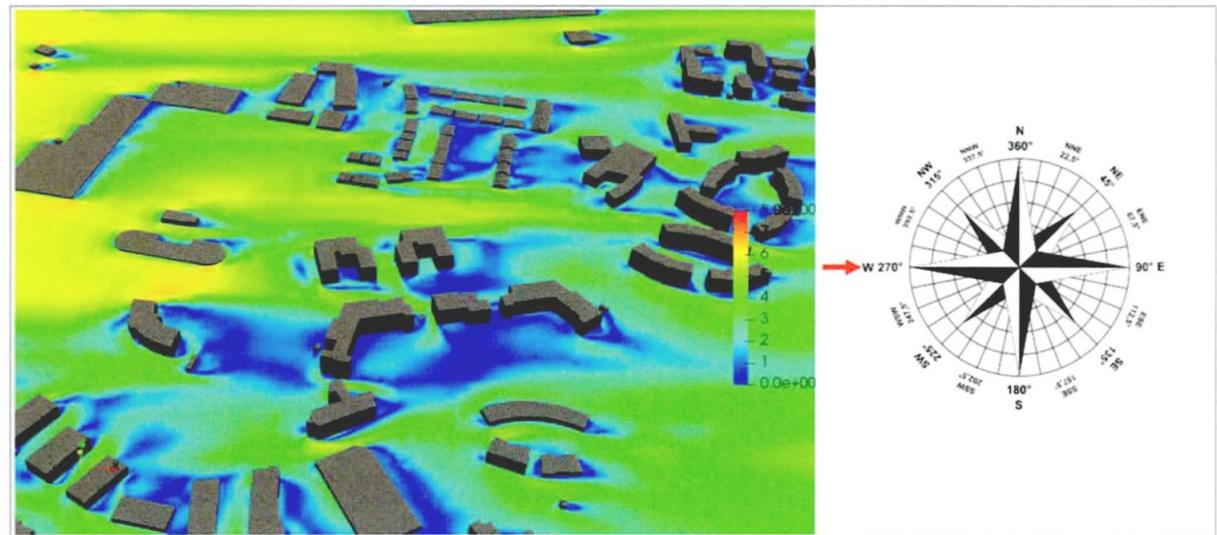
Figure 11-28: Pedestrian Level - Velocity Results at 1.5m above the ground - Wind Direction: 270°
